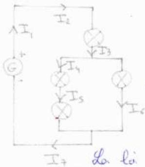
$I_1 = 200\text{mA}$  et  $I_4 = 120\text{mA}$
